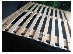
The front end is made out of a bed base bought in Jysk/Dänisches Bettenlager. For our purpose – since we are not very tall – we decided that the total length of the bed would be 178 cm, allowing the front seats to be in driving position. If you need a longer bed, you will have to push the seats forward, and if you also lets the back of the seat lean forward you may get 200 cm! The smallest Jysk bed base was enough for us – buy two if you want a longer bed.
