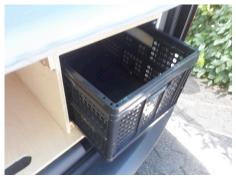
Both sections are closed with a piece of plywood plate in the front end to stabilize the construction, and to have a solid support for the front end of the bed.
