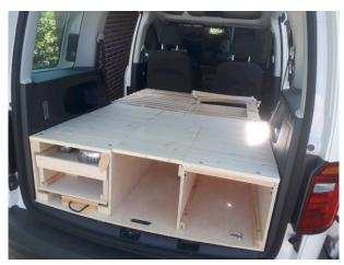
A bottom plate, 113 x 90 cm, (and most other parts) made of 12 mm plywood. Rear of the plate follows the form of the car.
