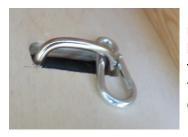
In case of a car accident, to keep the main part in place there are two safety locks in the back, and also one in the front end, fixing the box to the eyes in the bottom of the luggage room with carabiners.
